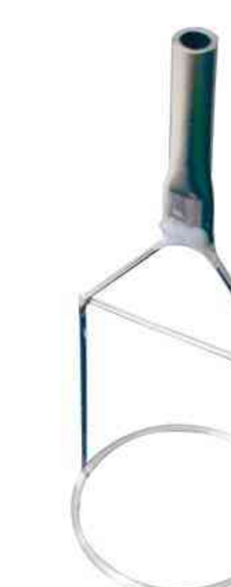
Platinum wire radius: 0.30mm Platinum ring radius: 9.85mm
